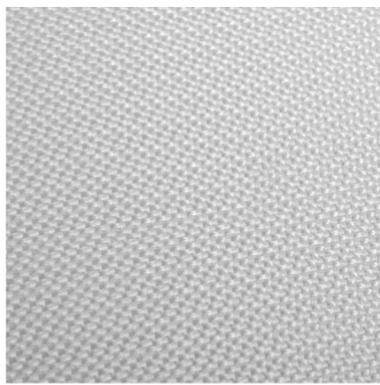
non-combustible, chemically neutral, absorbing water in minimum quantities and practically not subject to corrosion of water. It is resistant to mould, rotting and breakdown strength. It is certified by DNV. It is characterised of resistance on occurrence the high temperatures up to 450°C .
