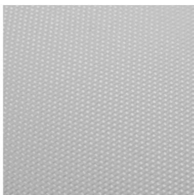
**Material:** glass fibre, aluminium coated
