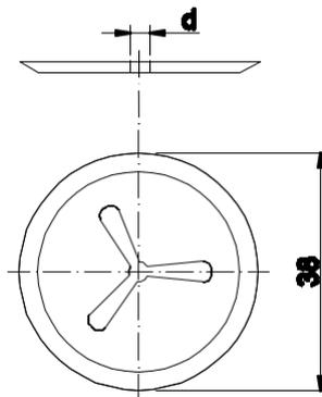
**Material:** galvanized steel ST, OC; stainless steel 1.4301
