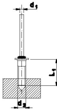
**Material:** copper covered steel, stainless steel 1.4301, screw galvanized, stainless steel
