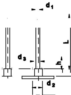
**Use:** assembling the insulation on aluminium surfaces in the marine and land industry. Bimetal pins are made of heat-sealable wire in diameter  $\varnothing 3\text{mm}$ .
