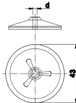
**Material:** galvanized steel ST, OC; stainless steel 1.4301
